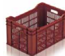
29049 (SN290401): 50 litres Ventilated stacking container Ext: 550 x 366 x 295mm Int: 518 x 333 x 260mm Wt: 2.02 Kg, colour: brown-red
